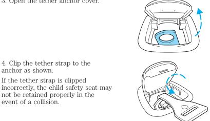
anchor as shown. If the tether strap is clipped
